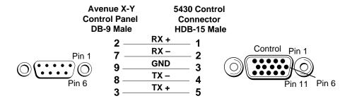
**Avenue X-Y Panel to Avenue Frame Control Cable Pinout**
