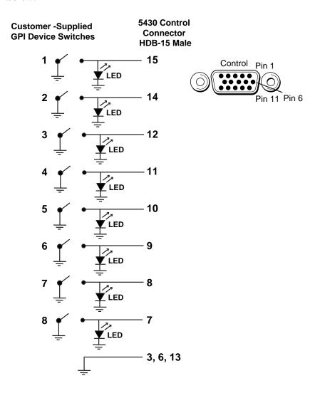
**GPI Control to Control Connector Pinouts**
