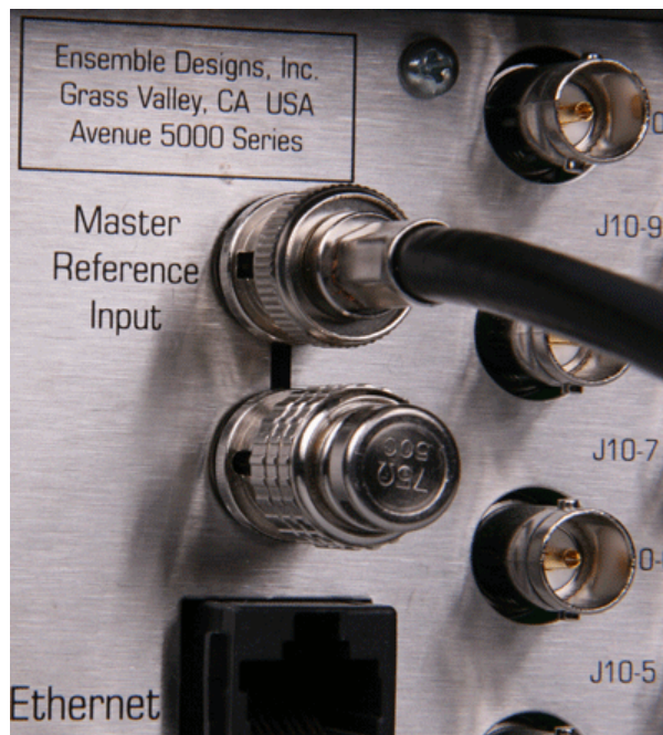
Connecting a Timing Reference to the Master Reference Input on the rear of the Avenue Frame. The loop through is terminated with a 75 ohm terminator.
