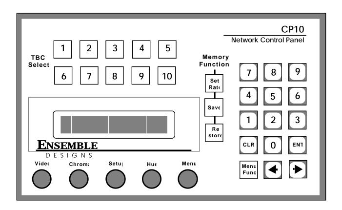
The CP10 control panel is designed to be used in edit suites and tape QC positions. It can access any of the machines connected to TC400D controllers in the system. CP10s and TC400Ds are connected in daisy chain fashion using ordinary modular telephone cable and connectors. At the beginning of a session machines are assigned to the ten TBC Select buttons using the alpha-numeric display.
