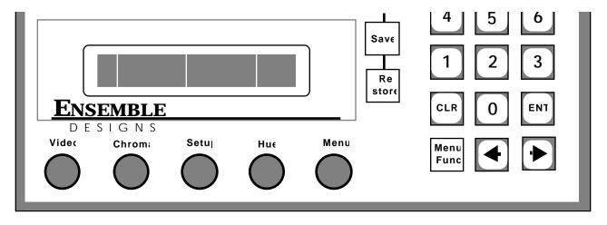
The firstset of functions: Adj Sync, Adj Subcarrier, Adj ColorFrame, Adj Y/C Delay, and Periph Enables, will be directed toward the TBC which is currently delegated on the TBC Select button group. Pgm Edit Port, Panel Name, Capture Enable, and AppleTalk are not affected by the TBC Select.
