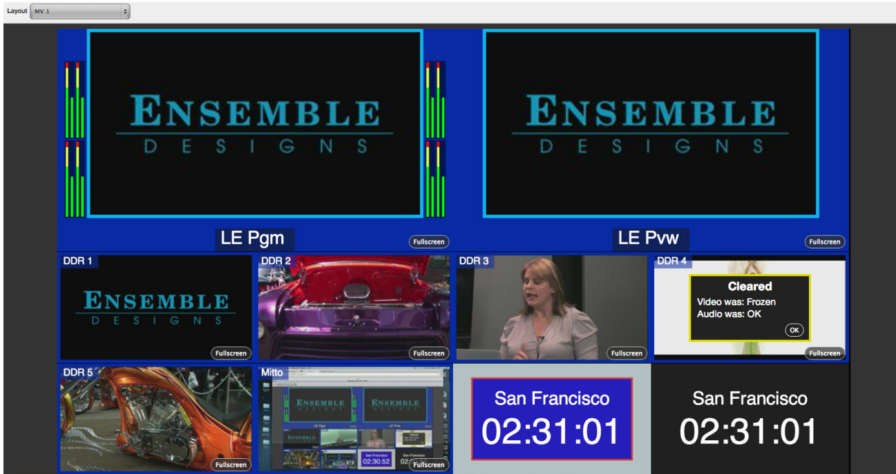
Multiviewer Control window showing a Fault Cleared Notice in the Cell for DDR 4
