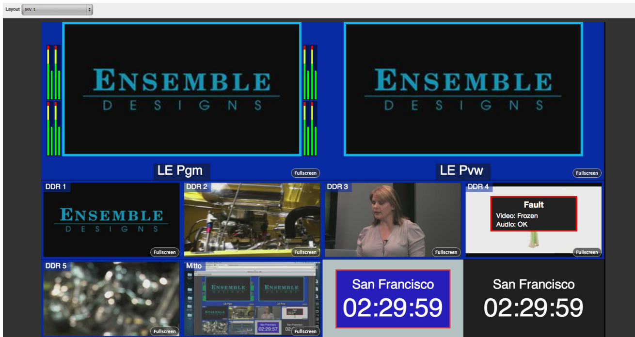
Multiviewer Control window showing a Fault Alarm in the Cell for DDR 4
