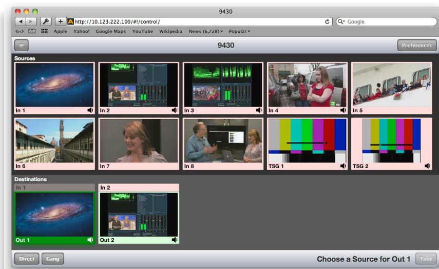
The 9430 Router control web interface showing video thumbnail images for 8 video inputs (In 1 through In 8), 2 test signal generators named TSG 1 and TSG 2, and 2 destinations named Out 1 and Out 2. In this example, In 1 is being routed to Out 1 while In 2 is being routed to Out 2.
