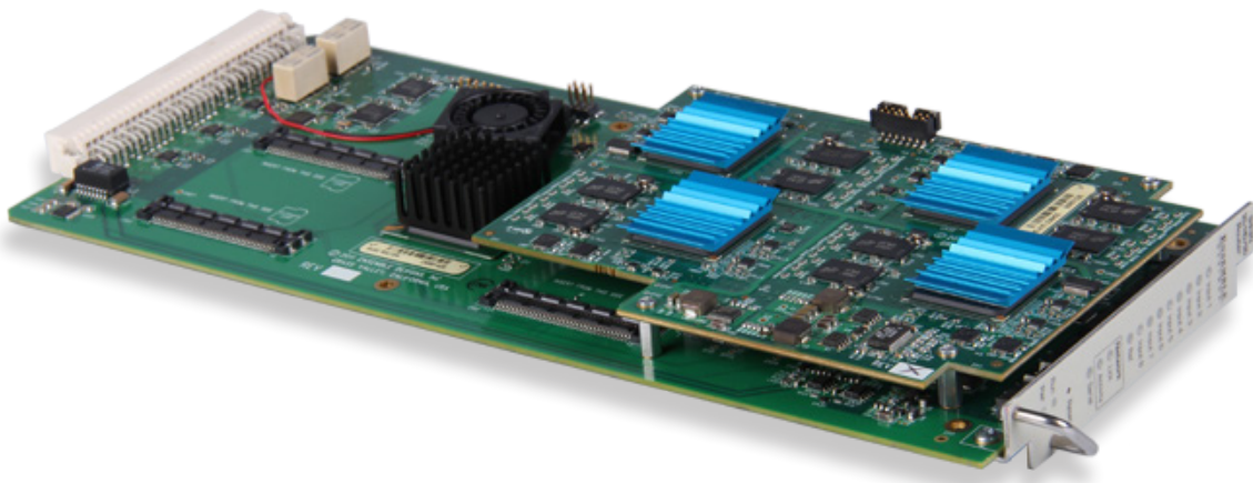
The P9425 Layering Engine consisting of the 9425 Layering Engine sub module mounted onto a 9430 Module
