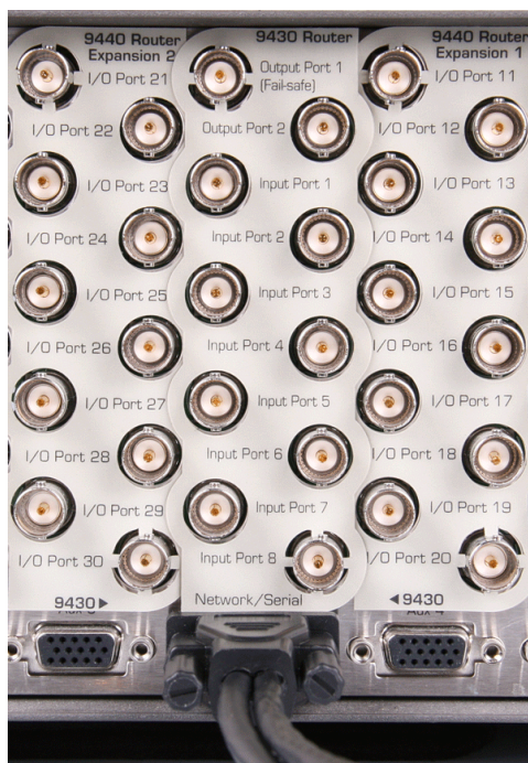
Adaptor "Y" cable (part number 23700040) for connecting the 9430 to RS-232 and 100 Mb Ethernet interfaces
