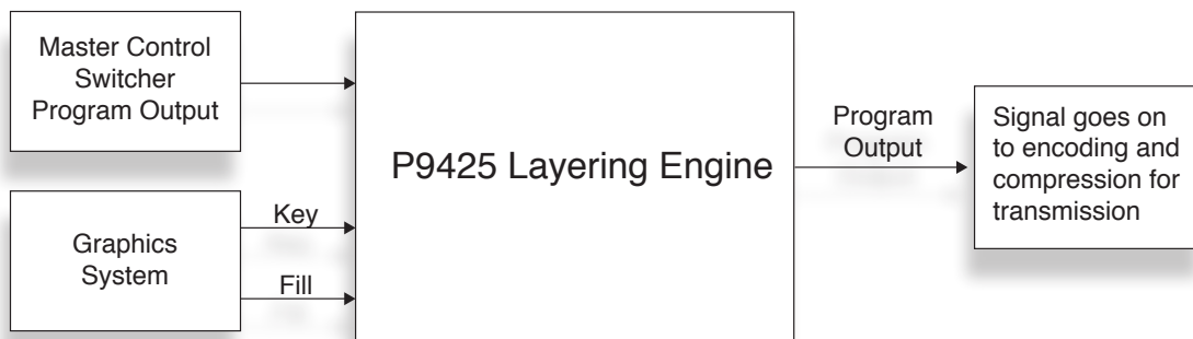
The Layering Engine configured for channel branding
